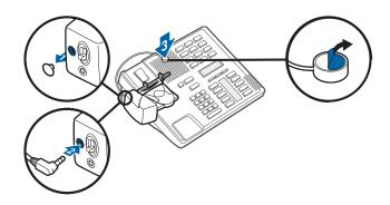
Use ringer microphone only when the telephone speaker is not located directly under the handset.
